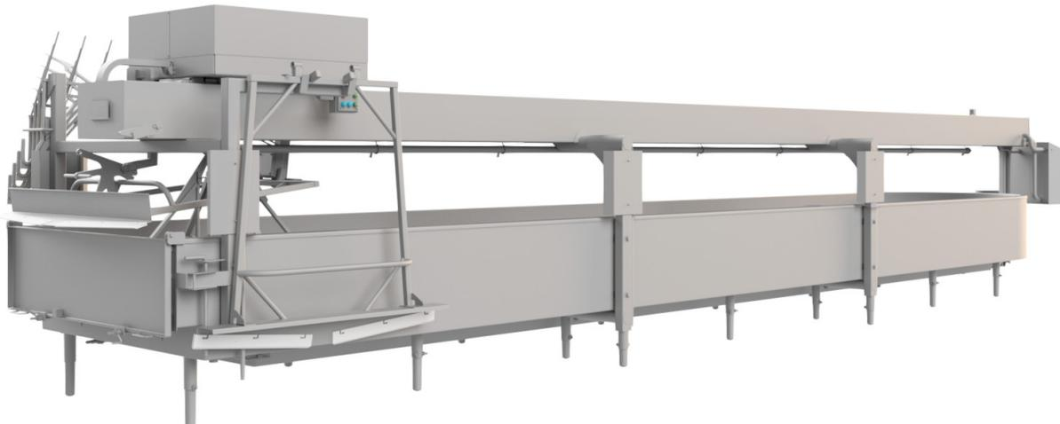
The RELCO® TRU-FINISH™ Curd Table is designed with the customer in mind to provide maximum flexibility. There are three distinct varieties offered: 1) The TRU-FINISH™ features our premium Rack and Pinion Drive, has an integrated drain screen, and is CIP-able. 2) The TRU-FINISH™ Classic is a chain-driven unit, has an integrated drain screen, and is CIP-able. 3) The TRU-FINISH™ Classic Lite is a chain-driven unit with removable drain screens and is our basic model.
